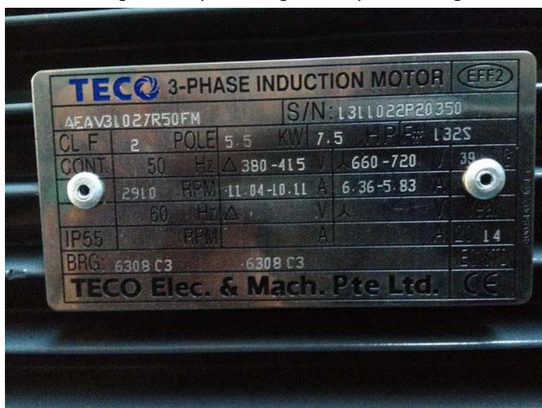
nameplate of the pump motor in this example
