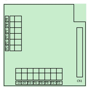
Connection diagram for EX-PG06 card adopting internal power supply
